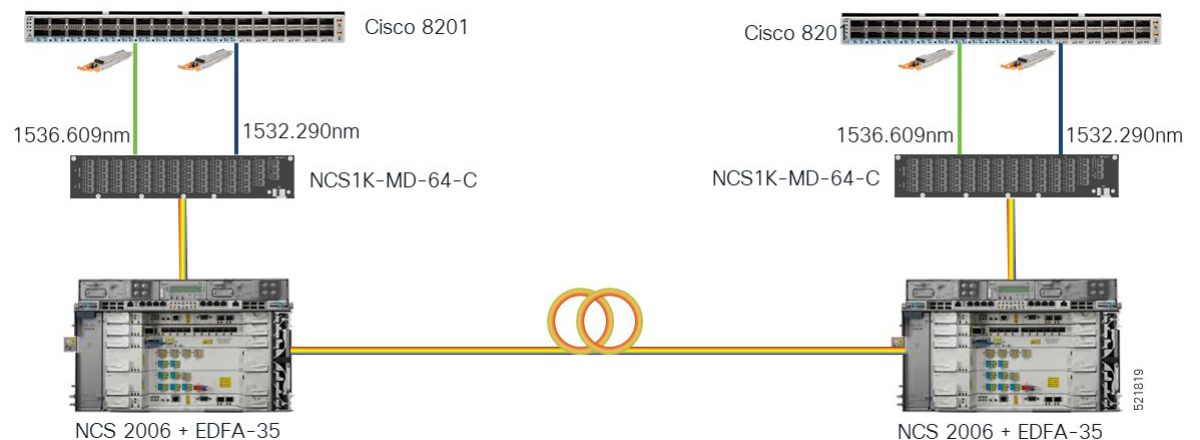
Figure 12: 400G-ZR P2P Short Haul Applications with Cisco NCS 2006
