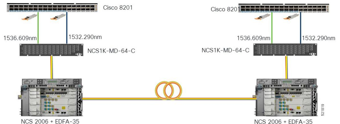
This diagram displays the wiring diagram for the metro/regional topology:
