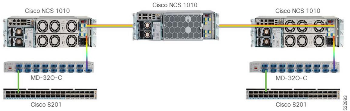
This diagram displays the wiring diagram for the point-to-point topology that uses NCS 1010 nodes.
