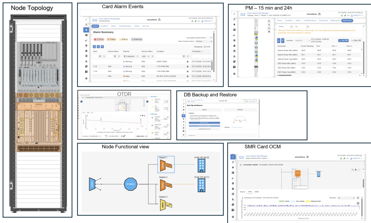
Figure 4: Cisco Optical Site Manager 2000 architecture and functions
