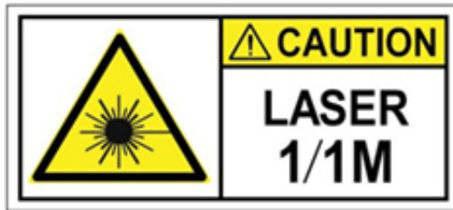
Figure 2: Class 1M Laser Product Label
