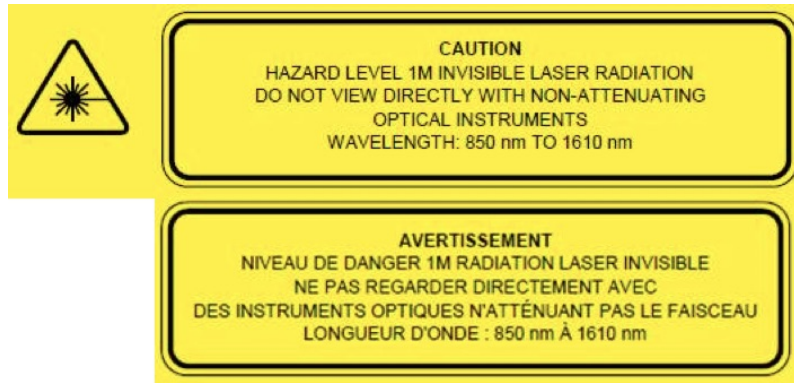
Figure 2: Class 1M Laser Product Label
