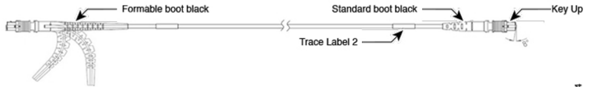
Figure 8: Cable with Formable Boot and Standard Boot
