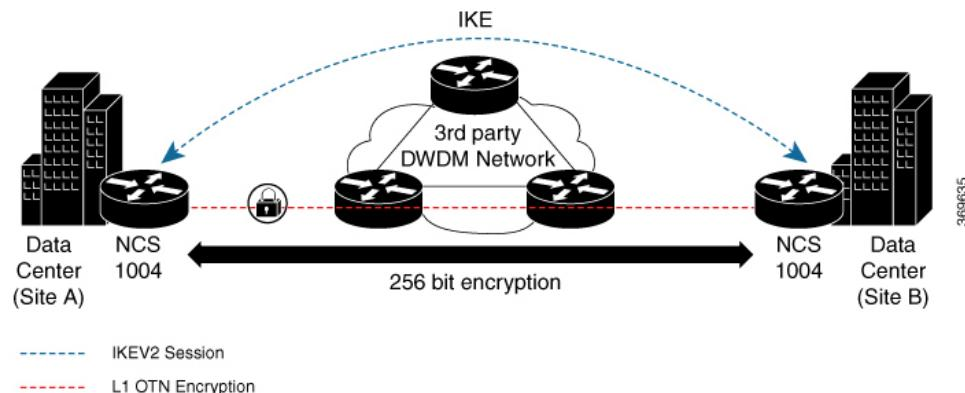
The recommended deployment is to have a single IKEv2 session running over a GCC2 channel per trunk port which creates the child SAs for each of the OTNSec controllers that are configured on the trunk port.
