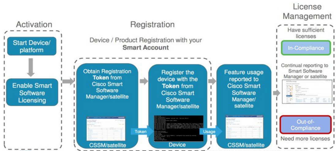
Figure 11: Smart Licensing Work Flow
