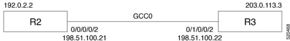
R2 is connected through GCC0 0/0/0/0 interface with IP address of 198.51.100.21 and R3 is connected through GCC0 0/1/0/0 with IP address of 198.51.100.22. The R2 and R3 devices are connected to external devices through management interfaces.
