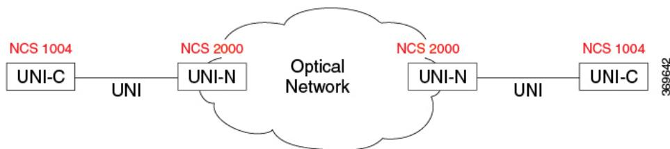
UNI-C is the client or packet or router node; for example, NCS 1004 nodes. UNI-N is the network or optical node; for example, NCS 2000 nodes.
