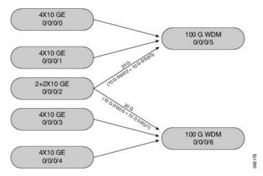
The following illustration describes the mapping of traffic from client to trunk ports for mixed mode configuration.
