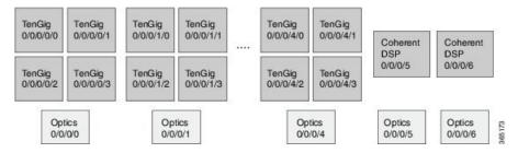
When the optics controller is shutdown, all four TenGig Ethernet controllers are shut down. Individual 10G port can be turned off from the TenGig Ethernet controller.
