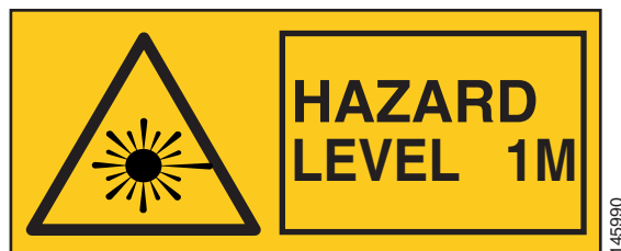
Figure G-8 Hazard Level Label
