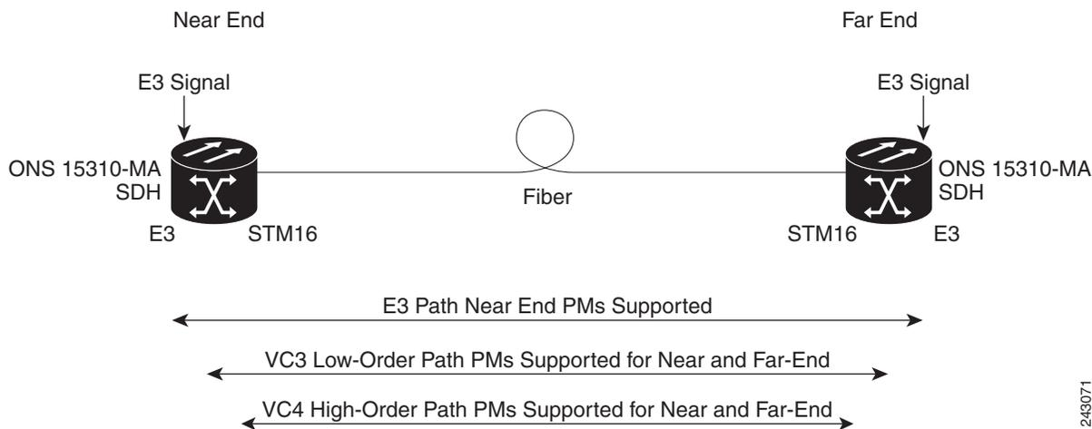
Figure 11-5 shows where overhead bytes detected on the ASICs produce performance monitoring parameters for the E3 ports.
