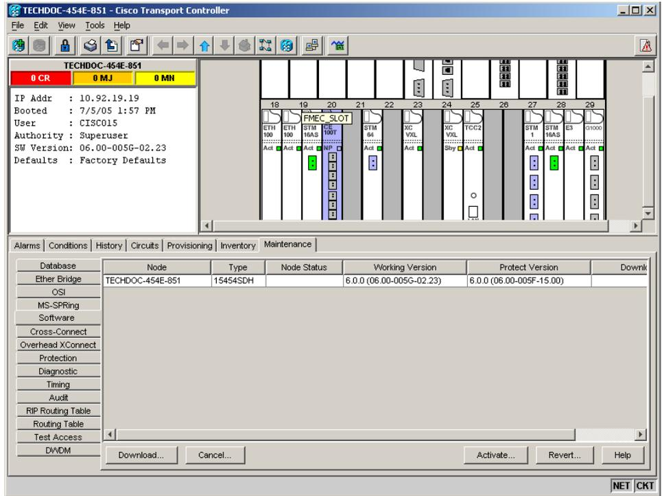
Select the Maintenance > Software tabs in network view to display the software versions installed on all the network nodes (Figure 8-2).
