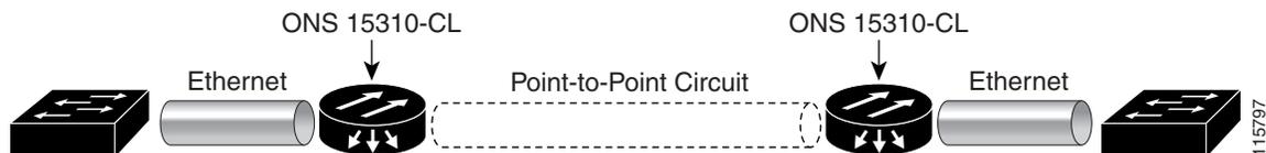
The CE-100T-8 cards allow you to provision and manage an Ethernet private line service like a traditional SONET line. CE-100T-8 card applications include providing Ethernet private line services and high-availability transport. It supports ITU-T G.707 and Telcordia GR-253 based standards for SONET.
