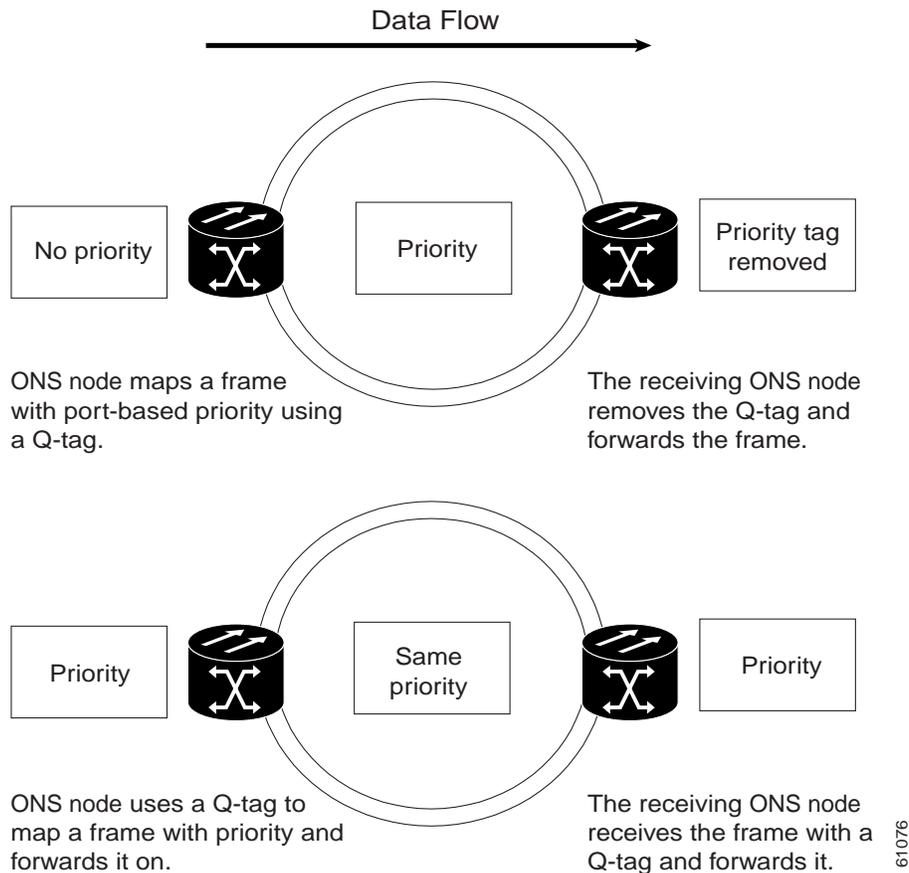
The ONS node uses a “leaky bucket” algorithm to establish a weighted priority. A weighted priority, as opposed to a strict priority, gives high-priority packets greater access to bandwidth, but does not totally preempt low-priority packets. During periods of network congestion, about 70 percent of bandwidth goes to the high-priority queue and the remaining 30 percent goes to the low-priority queue. A network that is too congested will drop packets.
