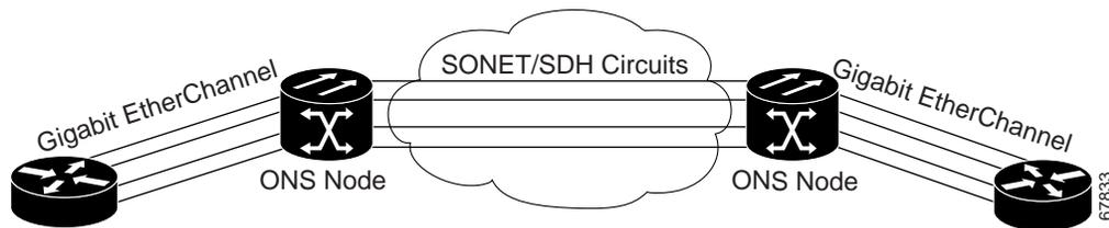
Although the G-Series cards do not actively run GEC, they support the end-to-end GEC functionality of attached Ethernet devices. If two Ethernet devices running GEC connect through G-Series cards to an ONS network, the ONS SONET/SDH side network is transparent to the EtherChannel devices. The EtherChannel devices operate as if they are directly connected to each other. Any combination of G-Series parallel circuit sizes can be used to support GEC throughput.
