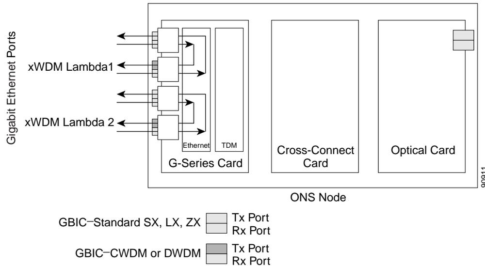
A G-Series card can be configured either for transponder mode or as the SONET/SDH default. When any port is provisioned in transponder mode, the card is in transponder mode and no SONET/SDH circuits can be configured until every port on the card goes back to SONET/SDH mode. To provision G-Series ports for transponder mode, refer to the *Cisco ONS 15454 Procedure Guide* or the *Cisco ONS 15454 SDH Procedure Guide*.
