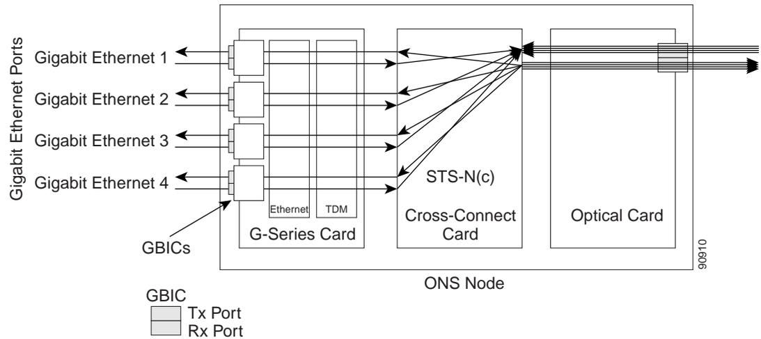
In transponder mode, the G-Series Ethernet traffic never comes into contact with the cross-connect card or the SONET/SDH network, but stays internal to the G-Series card and is routed back to a GBIC on that card (Figure 20-8).
