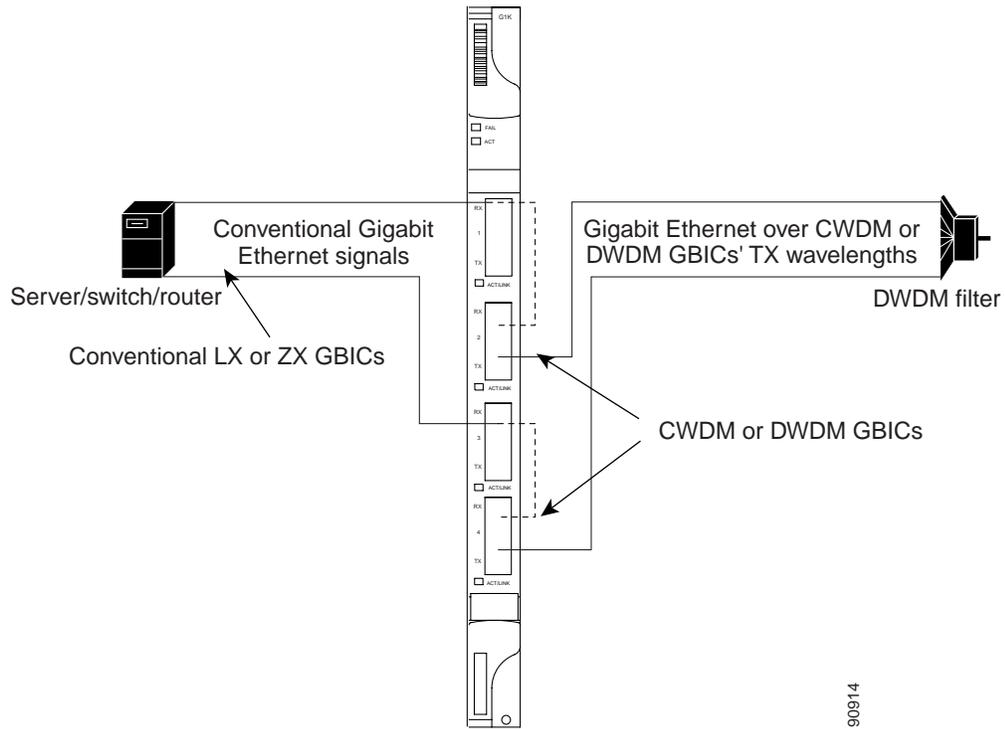
A G-Series card configured as a transponder operates quite differently than a G-Series card configured for SONET/SDH. In SONET/SDH configurations, the G-Series card receives and transmits Gigabit Ethernet traffic out the Ethernet ports and GBICs on the front of the card. This Ethernet traffic is multiplexed on and off the SONET/SDH network through the cross-connect card and the optical card (Figure 20-7).
