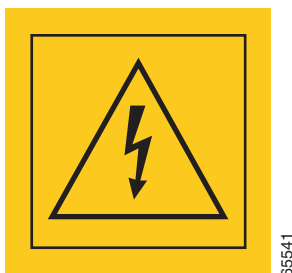
Figure 4-33 Electrical Energy Hazard Label
