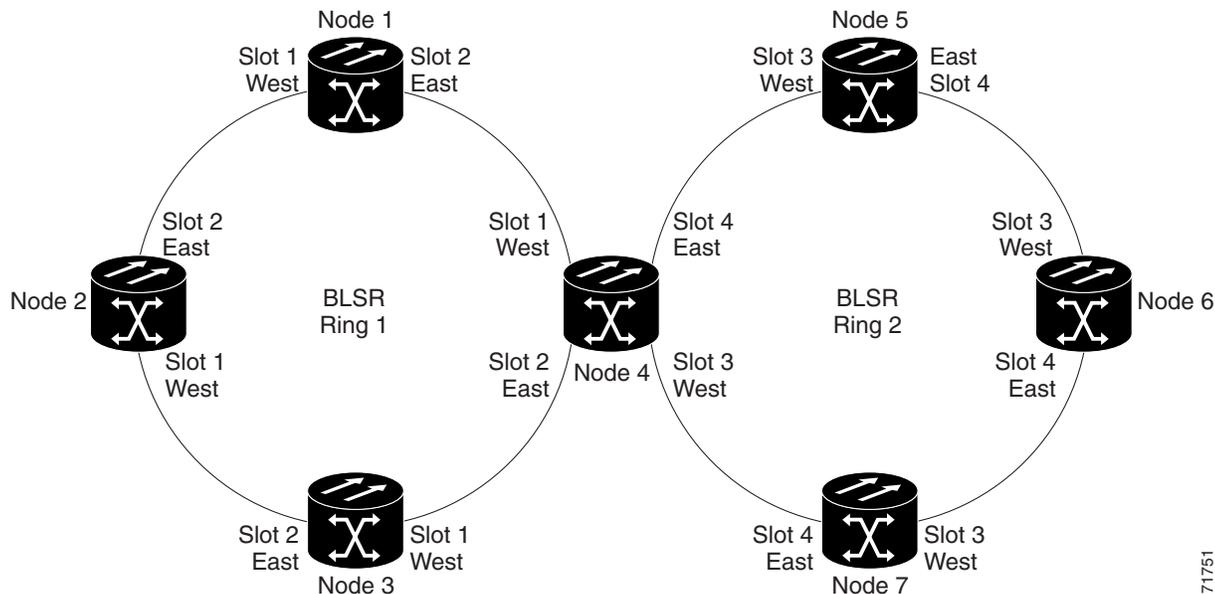
**Step 3** Attach fibers from the trunk cards in the subtending node to the BLSR trunk cards on its two neighboring BLSR nodes. In Figure 4-8, Node 4/Slot 3 connects to Node 7/Slot 4, and Node 4/Slot 4 connects to Node 5/Slot 3.
