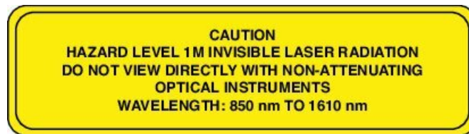
Figure 2: Class 1M Laser Product Label
