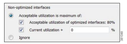
Example: There are two non-optimized interfaces: cr1.chi\_cr1.mia has a utilization of 60% and cr2.sjc\_cr2.okc has a utilization of 78%.
