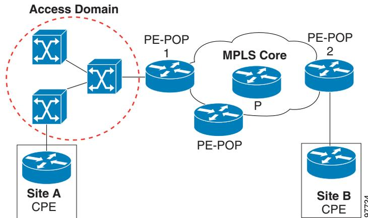
To create the NPCs for this network, first specify the link from the CPE at Site A to the PE-POP 1, and then one physical link for each intermediate switch between the CPE and PE-POP.
