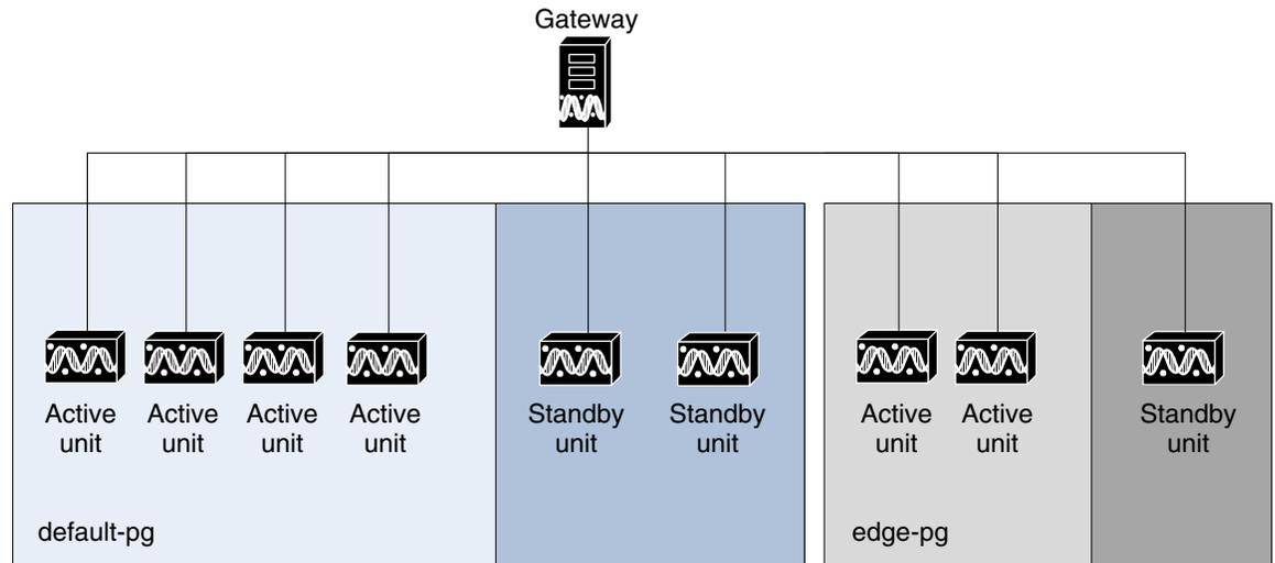
In the example configuration, when the gateway determines that one of the units in the protection group has failed, it notifies the standby unit of the protection group to immediately load the configuration of the failed unit. The standby unit loads the configuration of the failed unit, including all AVMs and VNEs, and functions as the failed unit. We recommend that you have two standby units per cluster. In this case, if a unit fails, another standby unit is still available.
