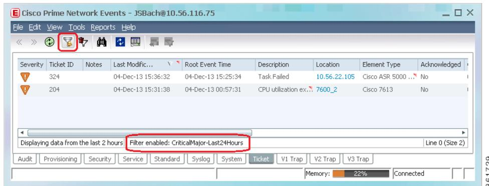
If the display is using a basic filter that was not saved, the client displays **Filter Enabled: Untitled**, as illustrated in Figure 13-6.
