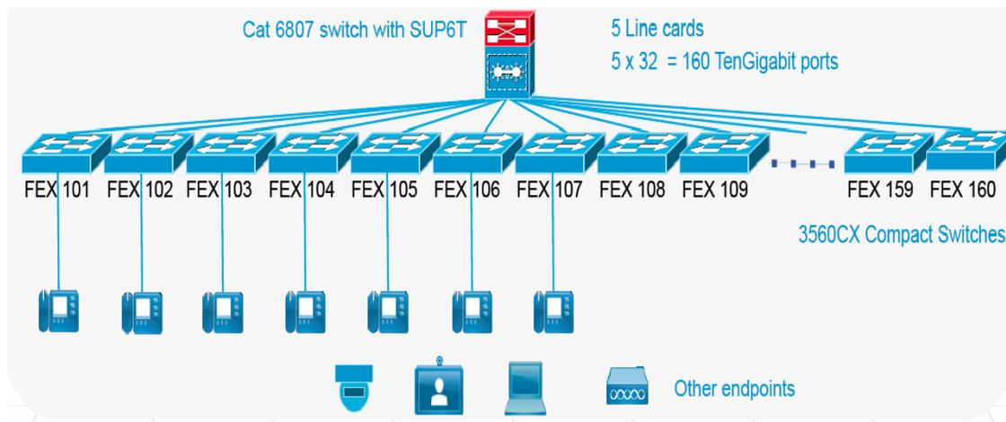
The sample Instant Access topology shown in Figure 48-1, includes a single catalyst 6807 chassis with 2 x SUP6T and 5 line cards. Each line card has 32 Ten Gigabit ports. Each port is connected to a FEX switch and the FEX switches are connected to different endpoints (IP Phones). The parent switch can be any supported switch as listed in [Supported Parent Switches](#).
