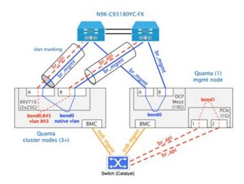
The management node uses the OCP Mezz NIC for br\_mgmt (2x10G on vlan 843) and the PCIe NIC for br\_api (2x1G on native vlan). The two br-api links of the management node are wired to the OOB switch.
