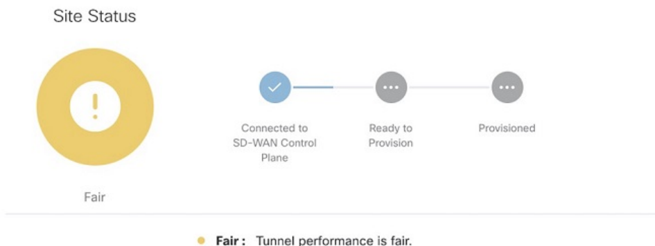
Figure 6: Connected to control plane but the tunnels are starting to degrade (fair)
