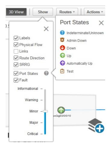
You can view either the alarm status or the primary state of the ports. For a list of the port primary state icons and a description of the states, see Port or Interface States.
