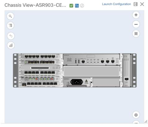
The Chassis View updates, displaying only the line card module that the port resides on and zooming in on it. The port pulsates in the Chassis View to help the user locate it. The badges that are displayed on the ports in this module indicate the primary status of those ports (see Port or Interface States, on page 15). Some elements may be surrounded by colored lines to indicate their state (out of service, preprovisioned, and so
