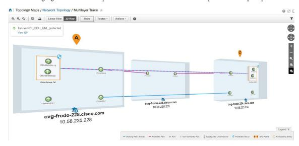
The following figure shows the simplified view of a circuit/VC with the expand and collapse options.
