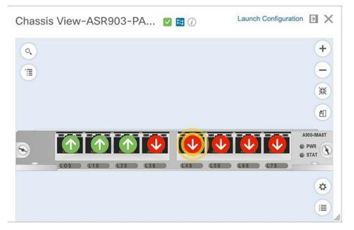
The Chassis View updates, displaying only the line card module that the port resides on and zooming in on it. The port pulsates in the Chassis View to help the user locate it. The badges that are displayed on the ports in this module indicate the primary status of those ports (see Port or Interface States, on page 15). Some elements may be surrounded by colored lines to indicate their state (out of service, preprovisioned, and so
