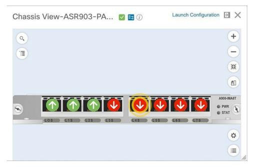
The Chassis View updates, displaying only the line card module that the port resides on and zooming in on it. The port pulsates in the Chassis View to help the user locate it. The badges that are displayed on the ports in this module indicate the primary status of those ports (see Port or Interface States, on page 15). Some elements may be surrounded by colored lines to indicate their state (out of service, preprovisioned, and so
