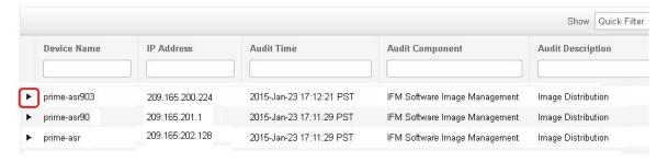
**Step 2** Expand an event drawer to get details about a device change. For example, if you expand the drawer highlighted in the above figure, you can see that the image listed in the job was successfully distributed to the device.
