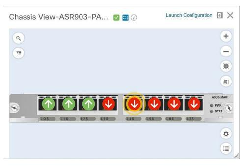
The Chassis View updates, displaying only the line card module that the port resides on and zooming in on it. The port pulsates in the Chassis View to help the user locate it. The badges displayed on the ports in this module indicate the primary status of those port (see Port or Interface States, on page 13). Some elements may be surrounded by colored lines to indicate their state (out of service, pre-provisioned, and so forth). To
