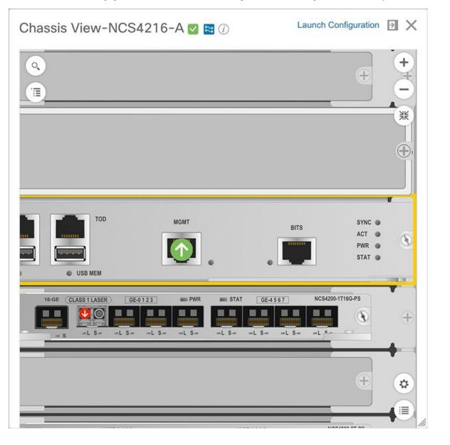
To customize the Chassis View so that alarm icons blink (to bring your attention them), click from the bottom right of the view, then check the **Enable Alarm Blinking** check box.
