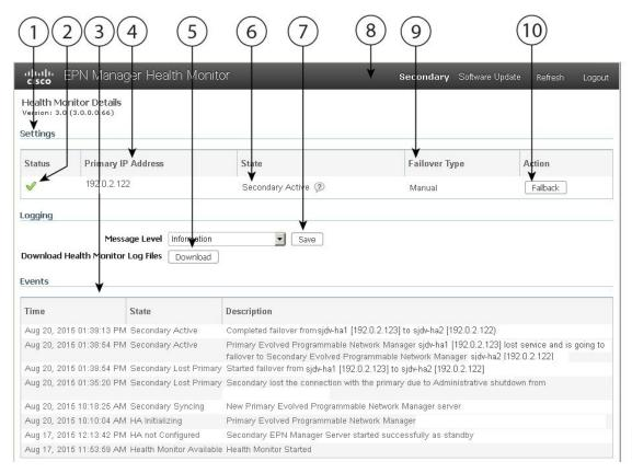
Settings—Displays the Health Monitor state and configuration detail in five separate sections.
