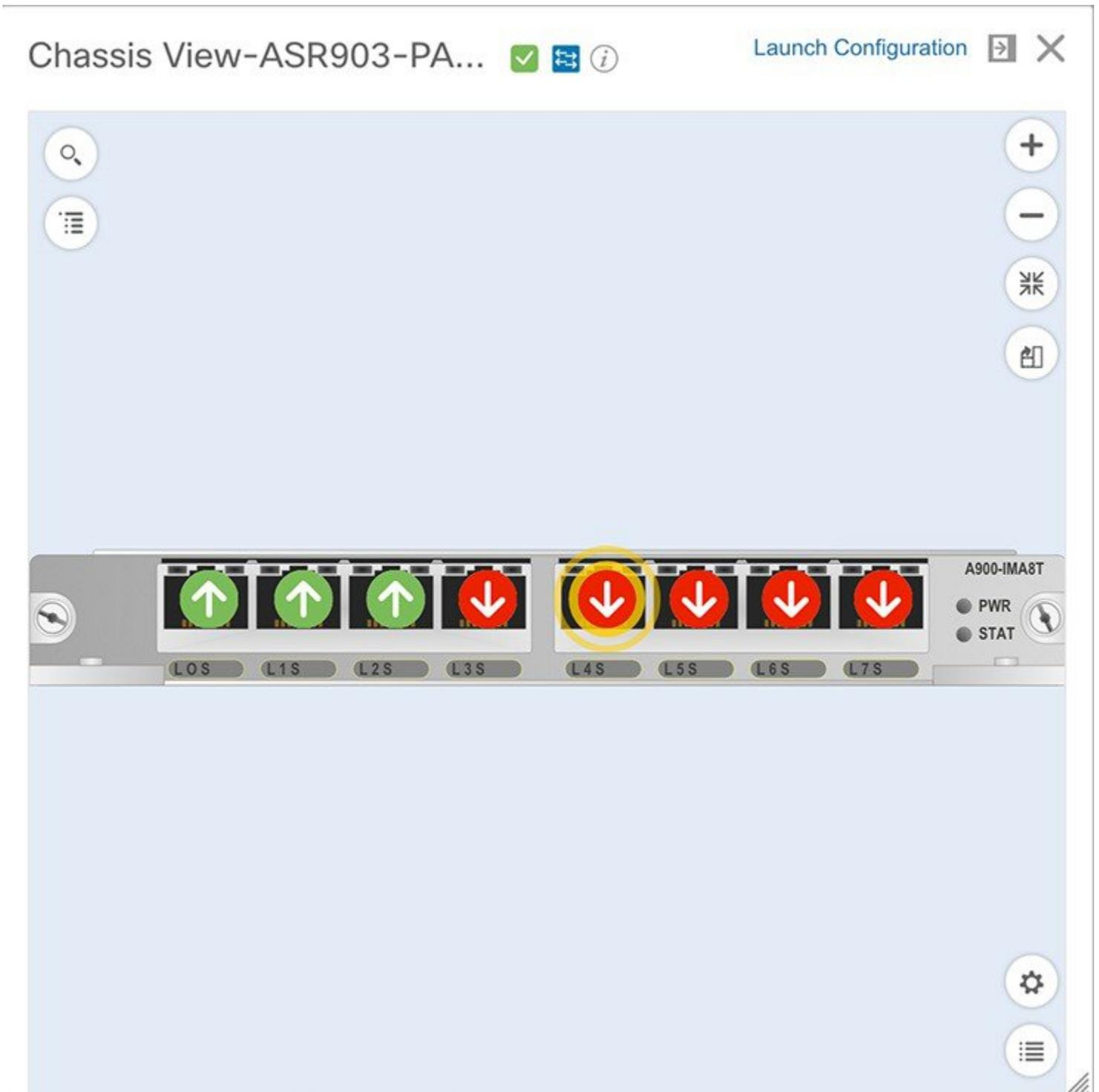
The Chassis View updates, displaying only the line card module that the port resides on and zooming in on it. The port pulsates in the Chassis View to help the user locate it. The badges displayed on the ports in this module indicate the primary status of those port (see [Port or Interface States](#), on page 16). Some elements may be surrounded by colored lines to indicate their state (out of service, pre-provisioned, and so forth). To
