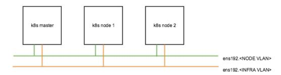
When creating a tenant cluster with ACI, you need to select an ACI profile. Cisco Container Platform uses the ACI profile to allocate the VLAN, pod subnet, service subnet, and multicase subnet.
