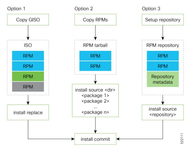
The software is split into modular blocks and the package manager infrastructure computes the dependencies between the blocks. Each block of software has a top-level package and various partition-level packages. Bug fixes that span multiple blocks may lead to creating multiple dependent packages that are built as part of earlier bug fixes.
