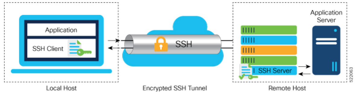
Figure 1: SSH Port Forwarding
