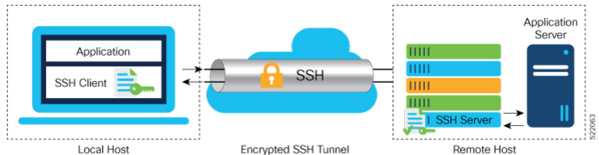
Figure 6: SSH Port Forwarding
