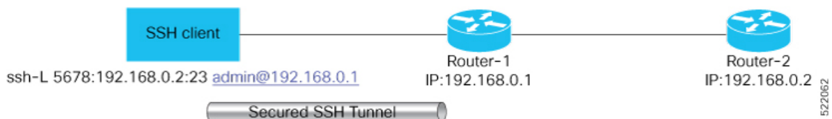
Figure 2: Sample Topology for SSH Port Forwarding
