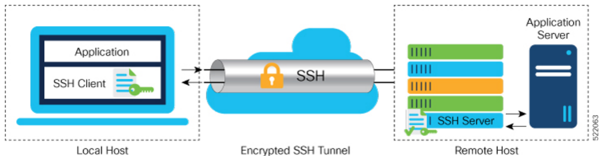
Figure 1: SSH Port Forwarding
