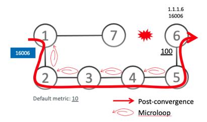
With microloop avoidance configured on Node1, a post-convergence path is computed and possible microloops on the post-convergence path for any destination are detected.
