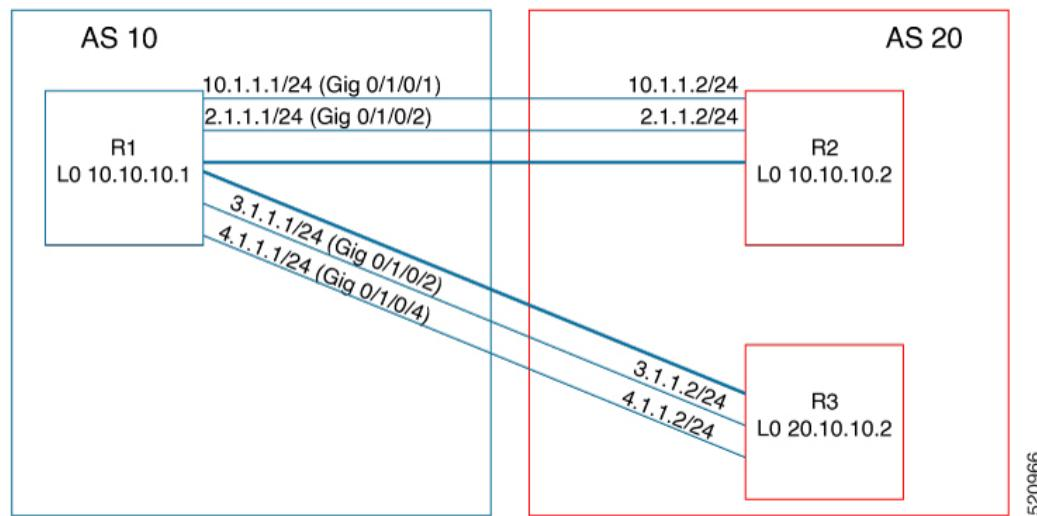
In this example, BGP-EPE peer SIDs are allocated from the default SRLB label range (15000 – 15999). The BGP-EPE peer SIDs are configured as follows:
