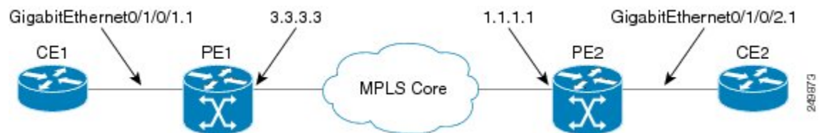
Figure 1: VPLS with BGP autodiscovery and BGP signaling
