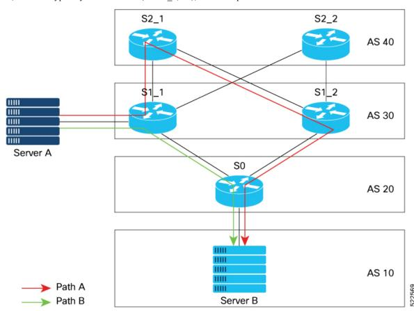
You may want to use Path A to reach the destination (via S1\_1, S2\_1, S1\_2, S0), for traffic engineering purpose. For example, Path A may be less congested and is better than Path B. To use Path A, you can replace the AS path values with one of the following options:
