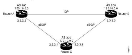
Here, Routers A and C and Routers B and C are running eBGP. Routers A and B are running an IGP (such as Routing Information Protocol [RIP], Interior Gateway Routing Protocol [IGRP], Enhanced IGRP, or Open Shortest Path First [OSPF]). The default distances for RIP, IGRP, Enhanced IGRP, and OSPF are 120, 100, 90, and 110, respectively. All these distances are higher than the default distance of eBGP, which is 20. Usually, the route with the lowest distance is preferred.
