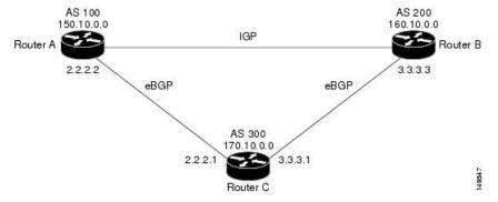
Here, Routers A and C and Routers B and C are running eBGP. Routers A and B are running an IGP (such as Routing Information Protocol [RIP], Interior Gateway Routing Protocol [IGRP], Enhanced IGRP, or Open Shortest Path First [OSPF]). The default distances for RIP, IGRP, Enhanced IGRP,
