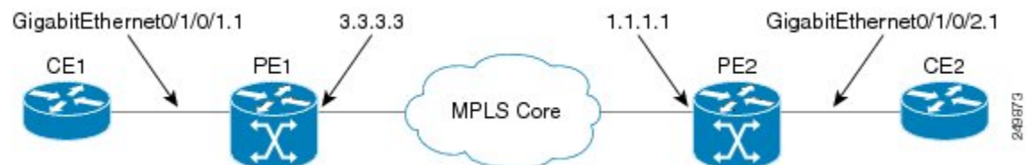
Figure 1: VPLS with BGP autodiscovery and BGP signaling
