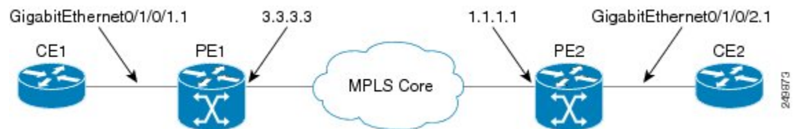
Figure 2: VPLS with BGP autodiscovery and BGP signaling
