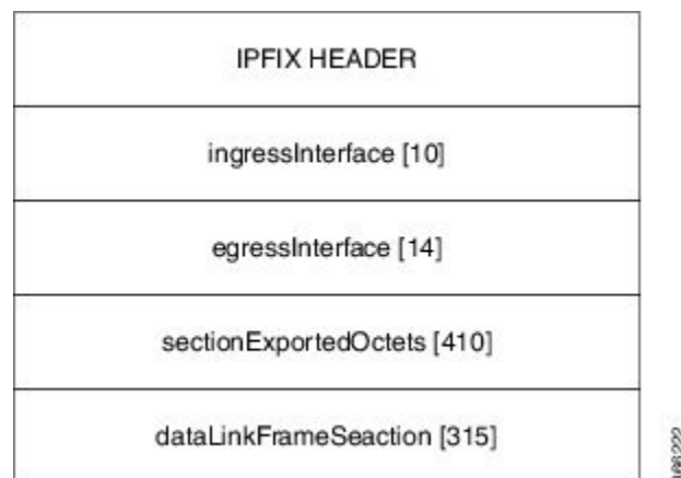
Figure 2: IPFIX 315 Export Packet Format
