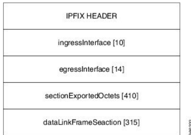
Figure 2: IPFIX 315 Export Packet Format
