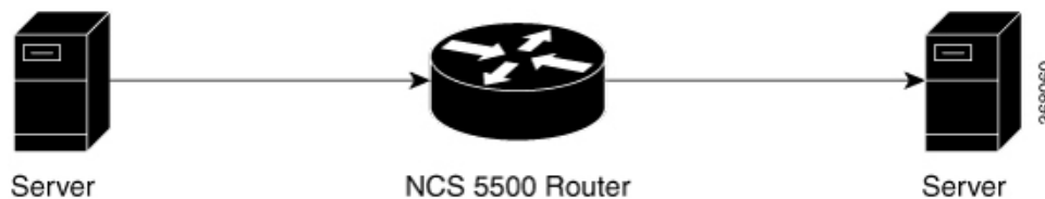
Figure 17: Topology for ERSPAN Egress Rate Limit
